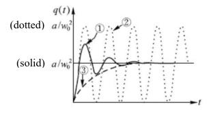
Fig. 7. Charge oscillation of RLC circuit with the DC power source (1)  $\beta = 0.2\omega_0$  (2)  $\beta = 0$  (3)  $\beta = \omega_0$
