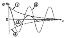
Fig. 5. Damped oscillation of charge in the RLC circuit with  $\delta = 0$ . ( $\beta^2 < \omega_0^2$ ) (DEnvelope of peaks (2)  $\beta = 0$  (without damping) (3)  $\beta = 0.2\omega_0$  (underdamped) (4) Envelope of valleys
