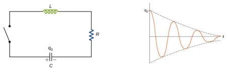
(a) RLC circuit (b) Damped oscillations of the capacitor charges Fig. 2. RC circuits with a two-pole switch
