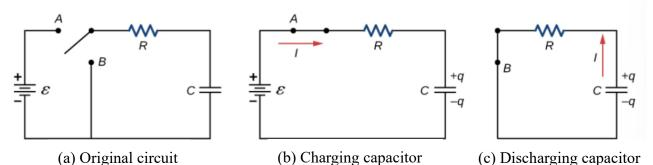
Fig. 1. RC circuits with a two-pole switch used to charge and discharge a capacitor.
