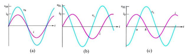
Fig. 11. Relationship between the current and (a) resistor (b) inductor (c) capacitor
