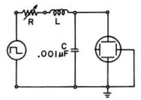
Fig. 14. Electrical circuit of the observation of charge oscillation in RLC circuit
