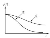
Fig. 6. Damped oscillation of charge in the RLC circuit. (D)Critical damping ( $\beta^2 = \omega_0^2$ ) (2)Overdamping ( $\beta^2 > \omega_0^2$ )
