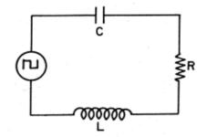
Fig. 8. Circuit diagram of RLC circuit with square wave source
