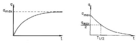
Fig. 3. Charging and discharging function of RC circuit
