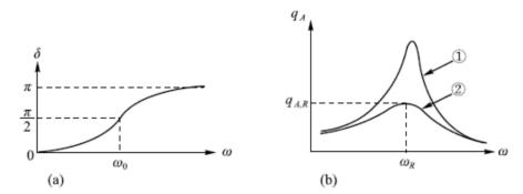
Fig. 9. Relationship between the driving frequency and (a) the phase and (b) amplitude, where  $\beta_1 < \beta_2$
