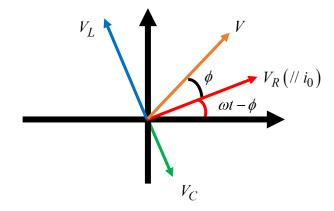
Fig. 12. Phasor diagram of the series RLC circuit.  $V_R, V_L, V_C$  are in phase with, 90° ahead of, and 90° behind the phasor of the current, respectively.
