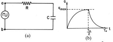
Fig. 4. (a) RC circuit with a square wave as the voltage source (b) charging and discharging behavior for the period  $T_0$  of the square wave larger than  $2\tau$ .
