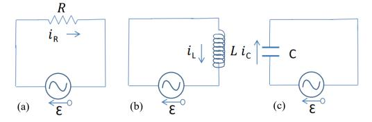
Fig. 10. Three simple AC circuits. (a) resistive load (b) inductive load (c) capacitive load
