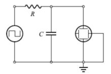
Fig. 13. Electrical circuit of the observation of charging and discharging the RC circuit
